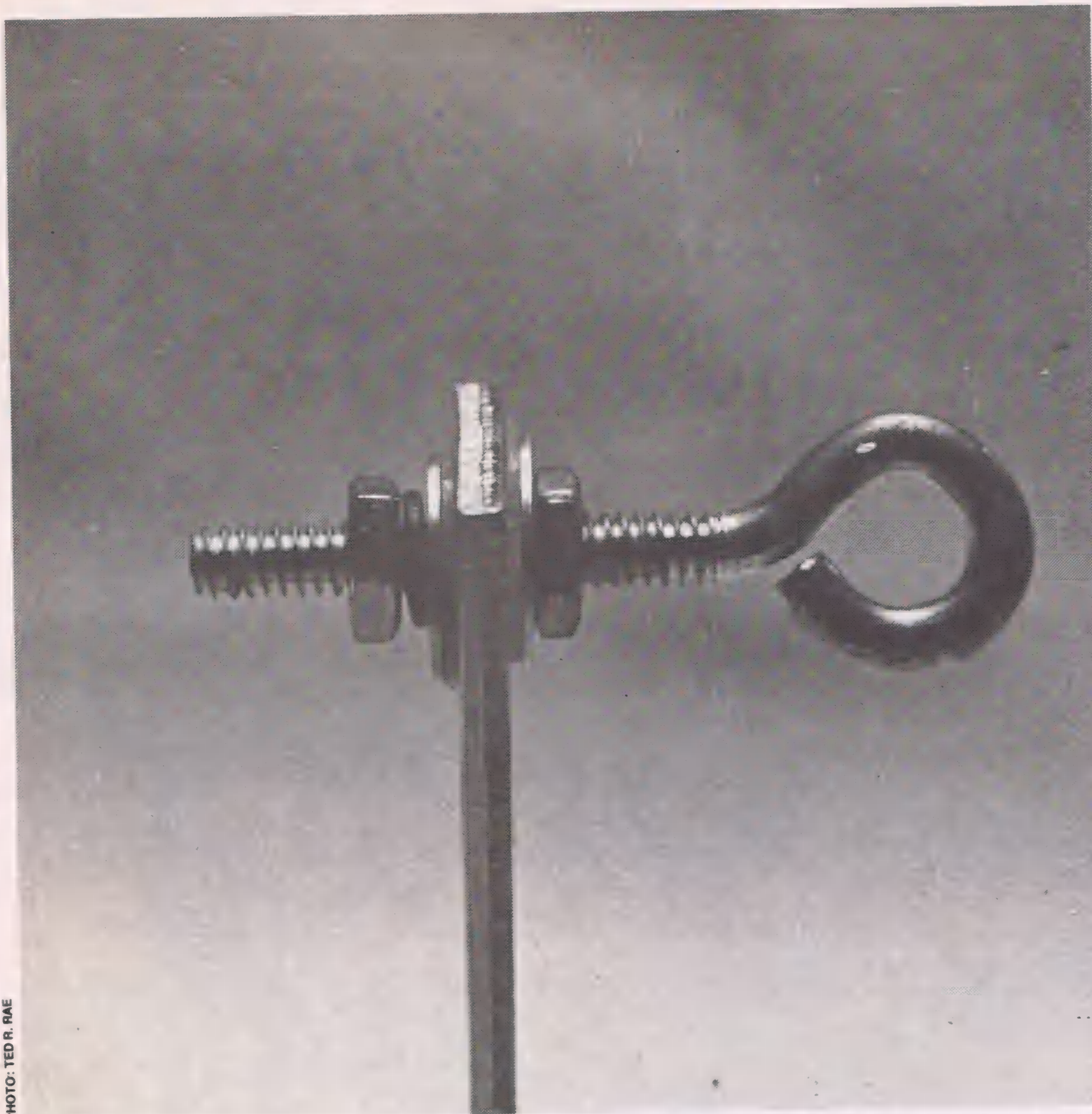
The support spindle assembly of the Simplified Aerial Brace showing the correct order of nuts and washers.
